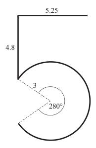
The shape has two straight sections of length 5.25 cm and 4.8 cm. The curved part is the arc of the major sector of a circle, radius 3 cm. The angle of the major sector is 280°.
