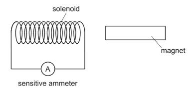
The magnet is pushed towards the solenoid. It accelerates, then moves at constant speed, then decelerates and stops inside the solenoid.
