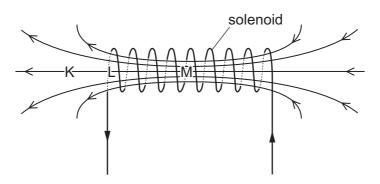
When the current in the solenoid is increased, where is there an increase in the magnetic field strength?
