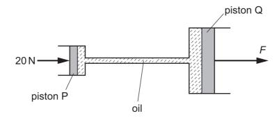
Piston P has an area of 5.0 cm<sup>2</sup> and piston Q has an area of 25 cm<sup>2</sup>.
