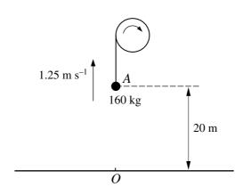
A load of mass 160 kg is pulled vertically upwards, from rest at a fixed point O on the ground, using a winding drum. The load passes through a point A, 20 m above O, with a speed of  $1.25 \,\mathrm{m\,s^{-1}}$  (see diagram). Find, for the motion from O to A,
