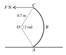
The diagram shows a uniform object ABC of weight 3 N in the form of an arc of a circle with centre O and radius 0.7 m. The angle AOC is 2 radians. The object rests in equilibrium with A on a horizontal surface and C vertically above A. Equilibrium is maintained by a horizontal force of magnitude F N applied at C in the plane of the object. Calculate F. [4]
