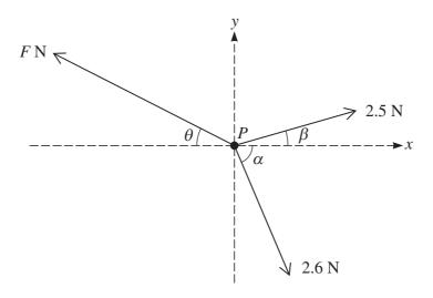
A particle *P* of mass 0.5 kg lies on a smooth horizontal plane. Horizontal forces of magnitudes *F* N, 2.5 N and 2.6 N act on *P*. The directions of the forces are as shown in the diagram, where  $\tan \alpha = \frac{12}{5}$  and  $\tan \beta = \frac{7}{24}$ .
