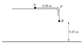
Particle A of mass 1.26 kg and particle B of mass 0.9 kg are attached to the ends of a light inextensible string. The string passes over a small smooth pulley P which is fixed at the edge of a rough horizontal table. A is held at rest at a point 0.48 m from P, and B hangs vertically below P, at a height of 0.45 m above the floor (see diagram). The coefficient of friction between A and the table is  $\frac{2}{7}$ . A is released and the particles start to move.
