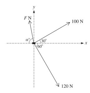
A small box of mass 40 kg is moved along a rough horizontal floor by three men. Two of the men apply horizontal forces of magnitudes 100 N and 120 N, making angles of 30° and 60° respectively with the positive x-direction. The third man applies a horizontal force of magnitude F N making an angle of  $\alpha$ ° with the negative x-direction (see diagram). The resultant of the three horizontal forces acting on the box is in the positive x-direction and has magnitude 136 N.
