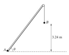
Particle A of mass 1.6 kg and particle B of mass 2 kg are attached to opposite ends of a light inextensible string. The string passes over a small smooth pulley fixed at the top of a smooth plane, which is inclined at angle  $\theta$ , where  $\sin \theta = 0.8$ . Particle A is held at rest at the bottom of the plane and B hangs at a height of 3.24 m above the level of the bottom of the plane (see diagram). A is released from rest and the particles start to move.
