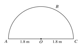
A uniform metal frame *OABC* is made from a semicircular arc *ABC* of radius 1.8 m, and a straight rod *AOC* with AO = OC = 1.8 m (see diagram).
