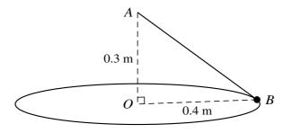
A small bead *B* of mass *m* kg moves with constant speed in a horizontal circle on a fixed smooth wire. The wire is in the form of a circle with centre *O* and radius 0.4 m. One end of a light elastic string of natural length 0.4 m and modulus of elasticity 42m N is attached to *B*. The other end of the string is attached to a fixed point *A* which is 0.3 m vertically above *O* (see diagram).
