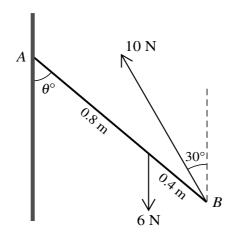
A non-uniform rod *AB* of weight 6 N rests in limiting equilibrium with the end *A* in contact with a rough vertical wall. AB = 1.2 m, the centre of mass of the rod is 0.8 m from *A*, and the angle between *AB* and the downward vertical is  $\theta^{\circ}$ . A force of magnitude 10 N acting at an angle of 30° to the upwards vertical is applied to the rod at *B* (see diagram). The rod and the line of action of the 10 N force lie in a vertical plane perpendicular to the wall. Calculate
