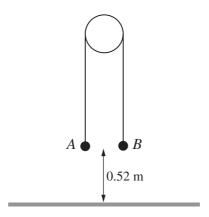
Particles A and B, of masses 0.3 kg and 0.7 kg respectively, are attached to the ends of a light inextensible string. The string passes over a fixed smooth pulley. A is held at rest and B hangs freely, with both straight parts of the string vertical and both particles at a height of 0.52 m above the floor (see diagram). A is released and both particles start to move.
