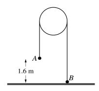
Particles A and B, of masses 0.35 kg and 0.15 kg respectively, are attached to the ends of a light inextensible string which passes over a fixed smooth pulley. The system is at rest with B held on the horizontal floor, the string taut and its straight parts vertical. A is at a height of 1.6 m above the floor (see diagram). B is released and the system begins to move; B does not reach the pulley. Find
