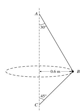
One end of a light inextensible string is attached to a fixed point *A*. The string passes through a smooth bead *B* of mass 0.3 kg and the other end of the string is attached to a fixed point *C* vertically below *A*. The bead *B* moves with constant speed in a horizontal circle of radius 0.6 m which has its centre between *A* and *C*. The string makes an angle of 30° with the vertical at *A* and an angle of 45° with the vertical at *C* (see diagram).
