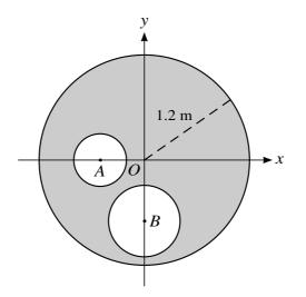
A uniform circular disc has centre *O* and radius 1.2 m. The centre of the disc is at the origin of *x*- and *y*-axes. Two circular holes with centres at *A* and *B* are made in the disc (see diagram). The point *A* is on the negative *x*-axis with OA = 0.5 m. The point *B* is on the negative *y*-axis with OB = 0.7 m. The hole with centre *A* has radius 0.3 m and the hole with centre *B* has radius 0.4 m. Find the distance of the centre of mass of the object from
