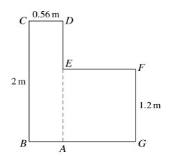
A uniform lamina is made by joining a rectangle *ABCD*, in which AB = CD = 0.56 m and BC = AD = 2 m, and a square *EFGA* of side 1.2 m. The vertex *E* of the square lies on the edge *AD* of the rectangle (see diagram). The centre of mass of the lamina is a distance *h* m from *BC* and a distance *v* m from *BAG*.
