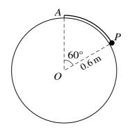
One end of a light inextensible string is attached to the highest point A of a solid fixed sphere with centre O and radius 0.6 m. The other end of the string is attached to a particle P of mass 0.2 kg which rests in contact with the smooth surface of the sphere. The angle  $AOP = 60^{\circ}$  (see diagram). The sphere exerts a contact force of magnitude R N on P and the tension in the string is T N.
