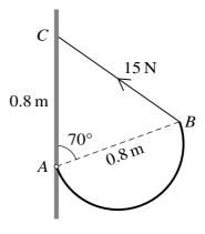
A uniform wire has the shape of a semicircular arc, with diameter AB of length 0.8 m. The wire is attached to a vertical wall by a smooth hinge at A. The wire is held in equilibrium with AB inclined at  $70^{\circ}$  to the upward vertical by a light string attached to B. The other end of the string is attached to the point C on the wall 0.8 m vertically above A. The tension in the string is 15 N (see diagram).
