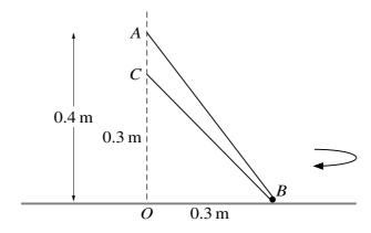
A light inextensible string passes through a small smooth bead B of mass  $0.4 \,\mathrm{kg}$ . One end of the string is attached to a fixed point A  $0.4 \,\mathrm{m}$  above a fixed point O on a smooth horizontal surface. The other end of the string is attached to a fixed point C which is vertically below A and  $0.3 \,\mathrm{m}$  above the surface. The bead moves with constant speed on the surface in a circle with centre O and radius  $0.3 \,\mathrm{m}$  (see diagram).
