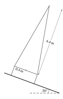
A uniform solid cone has base radius 0.4 m and height 4.4 m. A uniform solid cylinder has radius 0.4 m and weight equal to the weight of the cone. An object is formed by attaching the cylinder to the cone so that the base of the cone and a circular face of the cylinder are in contact and their circumferences coincide. The object rests in equilibrium with its circular base on a plane inclined at an angle of 20° to the horizontal (see diagram).
