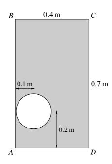
A uniform object is made by drilling a cylindrical hole through a rectangular block. The axis of the cylindrical hole is perpendicular to the cross-section *ABCD* through the centre of mass of the object. AB = CD = 0.7 m, BC = AD = 0.4 m, and the centre of the hole is 0.1 m from AB and 0.2 m from AD (see diagram). The hole has a cross-section of area  $0.03 \text{ m}^2$ .
