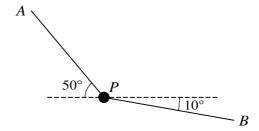
The diagram shows a small object P of mass 20 kg held in equilibrium by light ropes attached to fixed points A and B. The rope PA is inclined at an angle of 50° above the horizontal, the rope PB is inclined at an angle of 10° below the horizontal, and both ropes are in the same vertical plane. Find the tension in the rope PA and the tension in the rope PB.
