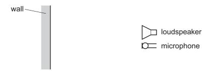
The loudspeaker makes a sound which is detected by the microphone.
