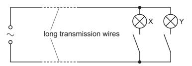
The identical lamps X and Y are connected to a low voltage a.c. power supply by high resistance transmission wires. Both lamps are switched on.
