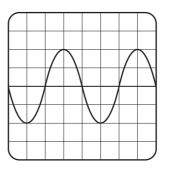
The coil now speeds up and rotates twice as fast.
