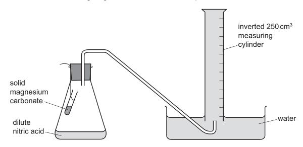
50 cm³ of dilute nitric acid was added to the conical flask. The contents of the test-tube were released, allowing the solid magnesium carbonate to mix with the dilute nitric acid. A stop-clock was started and the volume of gas collected in the inverted measuring cylinder was measured every 10 seconds for 80 seconds.
