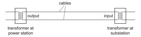
The power at the output of the transformer at the power station is 400 MW.
