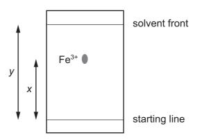
To make the spot containing  $Fe^{3+}(aq)$  more visible, the paper is sprayed with aqueous sodium hydroxide so that a precipitate of iron(III) hydroxide forms.
